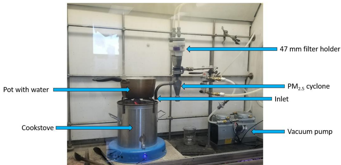
Figure 2.2.1 Experimental set-up for fine particulate matter collection with key instruments and parts labeled. This image features an African Clean Energy One cookstove following the Water Boiling Test protocol (modified image from Isenor, B.H.).
