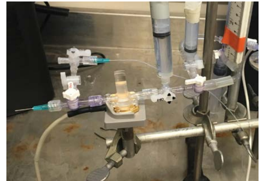
Figure 1.3: PowerLab Pressure transducer. This sent the signal to the transformer box to the LabChart8 on the computer.
