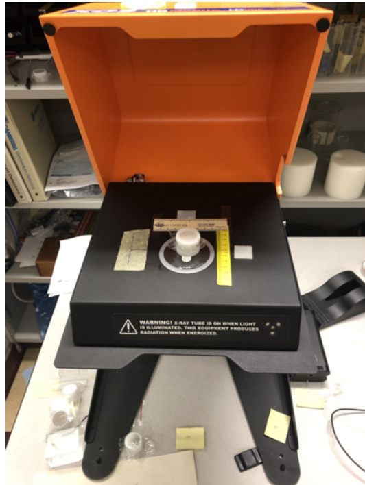
Figure 2.2: HD Mobile X-ray fluorescence system with okra sample on the measuring platform.
