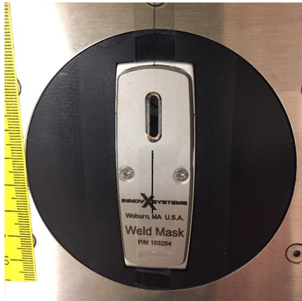
Figure 3: The weld mask configuration showing the location where samples are placed.
