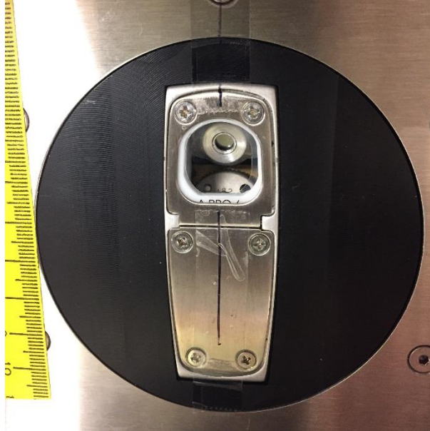
Figure 2: The open beam configuration showing the location where samples are placed.
