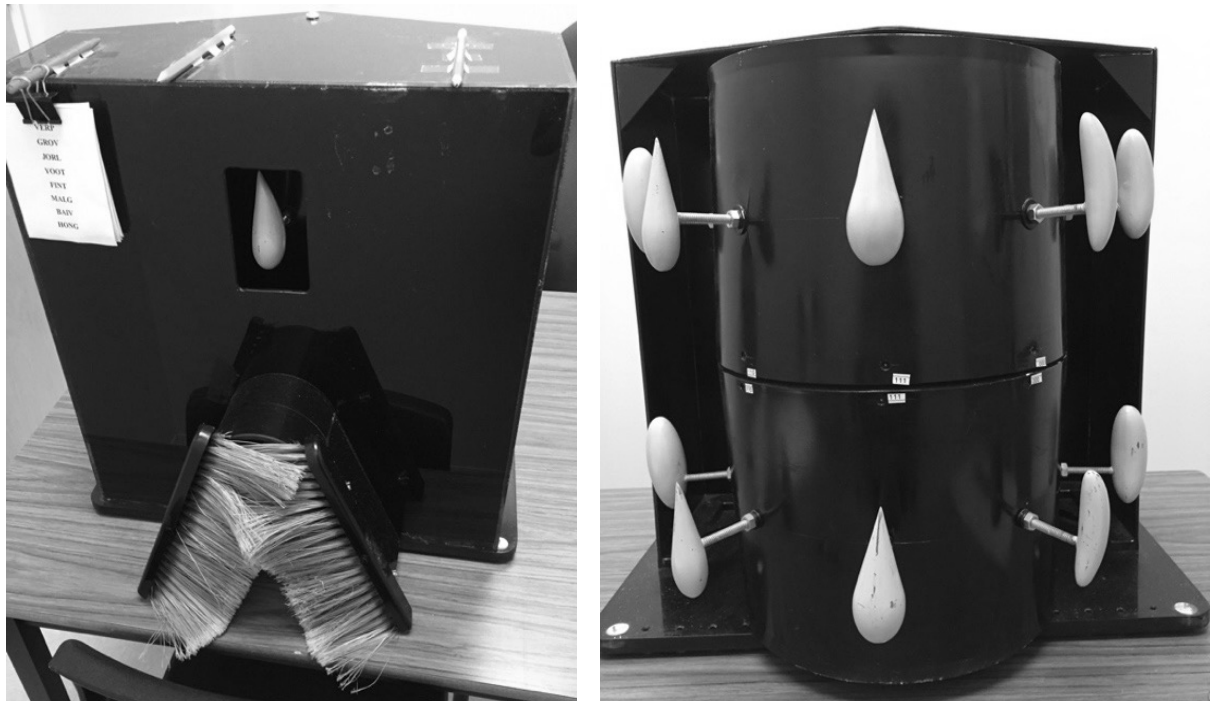
Figure 1. Apparatus used. Left: Participant viewpoint. During visual encoding and identification trials, objects appeared in the top window, while in haptic encoding and identification trials, participants reached into the bottom opening which concealed any view of the object being grasped. In the top left, a card displaying the eight non-word labels was placed in participants' field of vision. Right: experimenter view, showing identical object sets attached to the central cylinders of the apparatus.
