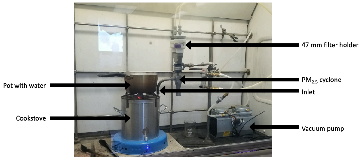
Figure 2.2.1. Particulate matter collection set-up. This labelled set up shows collection of PM 2.5 using the African Clean Energy One cookstove following the Water Boiling Test protocol.
